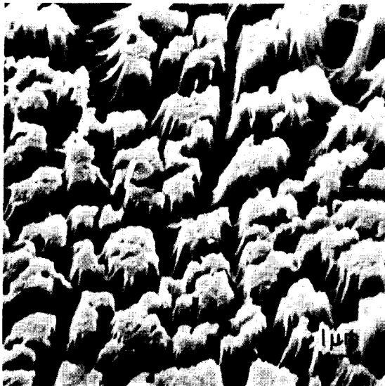
Figure 4 Polyethylene from aluminium anodized in 4% phosphoric acid at 20 V for 60 min at 24°C. [Reproduced from Wake, W. C. 'Adhesion and the formulation of adhesives', Applied Science, 1976, p 70 by permission of Applied Science Publishers Ltd, Barking ©]
